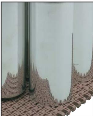
**uni M-SNB M3:** Suitable for upside-down can transport applications, PET bottles, and items with fragile surfaces. It has heavy duty edges to withstand wear. This belt is available with prepolished surface for raw-edge can applications.
