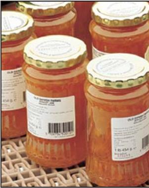
The special surface profile of the belt is designed to give minimum resistance against products and wearstrips. The open design is easy-to-clean.
