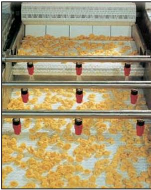
The open surface versions of uni Light are used e.g. where drainage or airflow through the belt is required.
