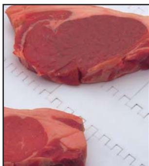
The uni MPB Closed is used for meat chopping and cutting operations. It has a smooth surface preventing dirt from getting caught between the hinges. A very smooth surface means optimum cleanability.
