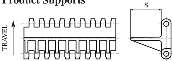
uni OPB product support with reinforcement ribs
