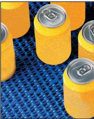
The patented surface pattern reduces the friction as well as the dirt and the aluminium oxide remnants on the belt.
