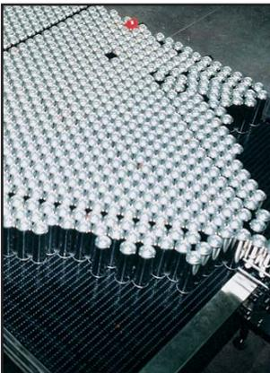
The very smooth surface makes uni SNB M1 well suited for accumulation systems with back line pressure.
