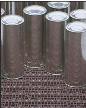
uni L-SNB is a strong belt for pasteurizers as it is able to withstand the extreme conditions in an application with different heat zones.
