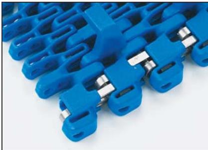
**uni Flex SNB-WT:** Standard radius fitted with reinforcement links and steel pins. Integral moulded edge wearpart. Integral underside tab (S-Tab.)
