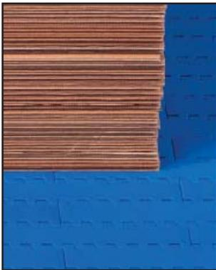
uni QNB has become very popular in the corrugated and cardboard industry. Its flat, solid, smooth and even surface increases safety for the workers and eliminates sheet warp, pressure damage and marks on the lower sheets. A steady run eliminates stack tippage.
