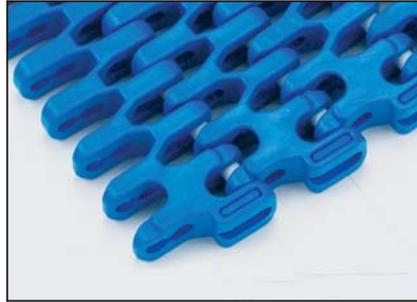
**uni Flex SNB-CR:** Tight radius. Min. inside radius from 1.5 x belt width. 47% open hygienic solid grid surface.
