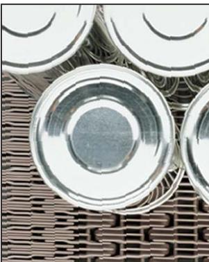
uni L-SNB is also available in a rib version that can be used with finger plates and thus is suitable for product transfer applications.
