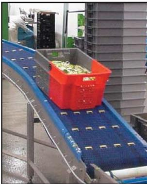
uni Flex SNB-W with reinforcement links and rubber supports.
