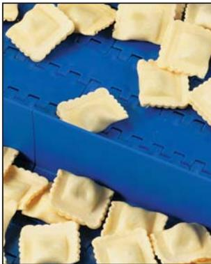
uni CNB with closed surface is suitable for light food applications.
