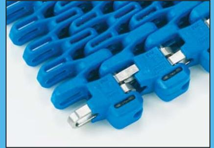
**uni Flex SNB-W:** Standard radius fitted with reinforcement links and steel pins. Integral moulded edge wearpart.
