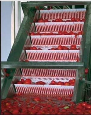
Product supports and side guards in different heights enable e.g. inclined transport. Various open versions are suitable for applications with drainage or air flow.
