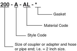
If coupling is a reducing size, the coupler or adapter is the first size (i.e. 4030-C is 4 inch coupler to 3 inch hose shank.)
